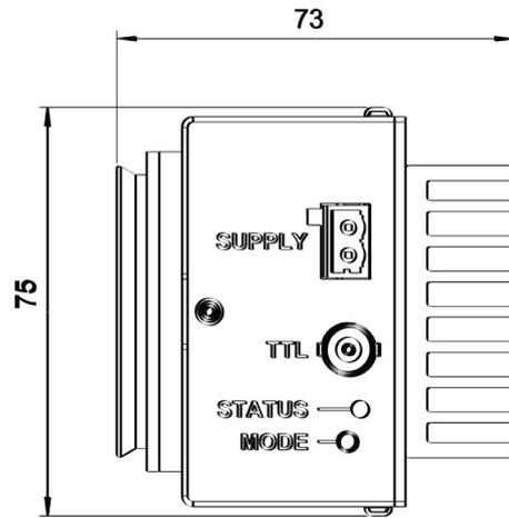
Top view luxyr LED NANO | Dimensions in mm
