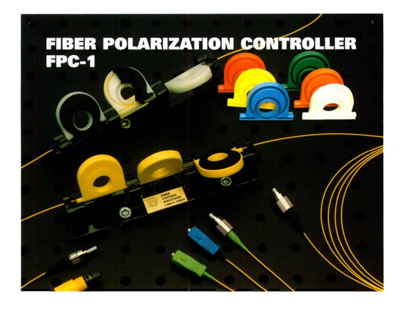
FIBER CONTROL INDUSTRIES polarization controller's unique user-friendly design utilizes stress-induced birefringence to alter and control the state-of-polarization of light in single-mode fibers. Each paddle acts as a fractional waveplate. Complete coverage of the Poincaré sphere and polarization control is provided by adjusting the angles of the paddles.
