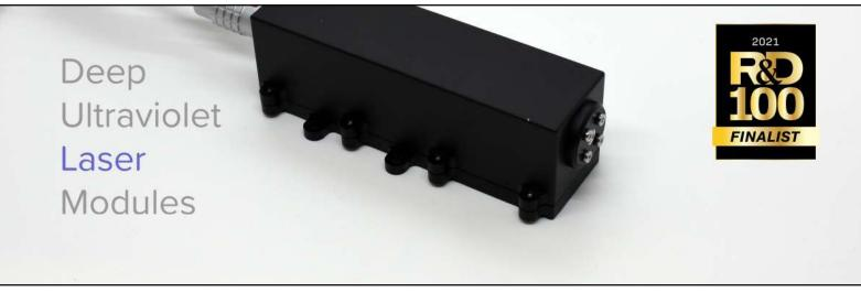
Model 261 lasers are the worlds only deep ultraviolet diode laser modules. They are OEM components which provide greater than 10 mW of continuous wave output at 261 nanometers. Their extremely compact size, wide operating temperature range, and low divergence output beam enables easy integration into fixed, portable, and handheld systems.
