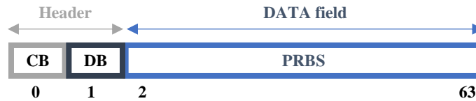
Figure 39: PRBS frames sent during the PRBS Alignment Sequence (PAS).
