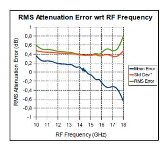
6. Measurements de-embedded for a probe inductance of 0.3 nH at both input and output.
