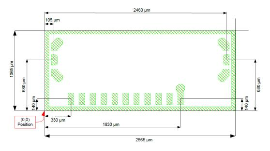
Chip Size = 2600 x 1100  $\mu$ m (2565 x 1065  $\mu$ m ± 5  $\mu$ m after dicing) DC Pads = 80 x 160  $\mu$ m, spacing = 70  $\mu$ m, top metal = Au RF Pads = 85 x 150  $\mu$ m, top metal = Au Chip Thickness = 100  $\mu$ m
