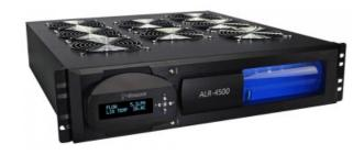
ALR-4500 is Koolance's highest performing ambient liquid cooling system. It can be oriented in horizontal or vertical orientations, and is rack-mountable. This model contains a large eight x 120mm fan aluminum radiator, providing roughly 4300W of cooling with a 25 °C ambient delta. Coolant flow rate, temperature, and reservoir level are monitored, and a USB port allows control and logging of most features using the Koolance System Monitor application.
