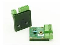
Koheron PDX10R is a logarithmic photodetector for free-space optical power measurements. In addition to two analog outputs log(A) and log(B), it provides the log-ratio log(A/B) with an adjustable offset and two gain settings (x1 and x10). The PDX10R provides a fully-analog solution for direct absorption measurement in spectroscopy setups.
