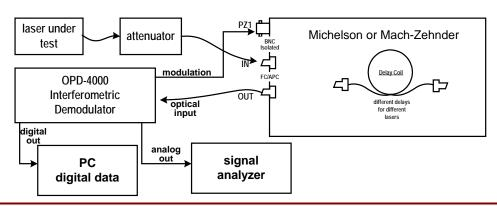
Laser under test is input to interferometer, which is set to the appropriate optical path mismatch by selection of the delay line which may be user installed or changed. OPD-4000 modulation output is applied to the PZ1 fiber stretcher input. OPD-4000 phase measurement output is selected as either digital or analog. Digital data is post processed. Analog data is available to signal made analyzer.
