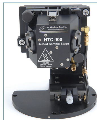
HTC-100 Heat Stage (Room Temp. to 300°C)
