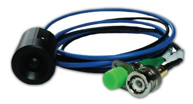
Our fiber coupled TERA15-FC antenna modules for 1560 nm laser wavelength are the unique solution for flexible and robust all-fiber THz-TDS systems. The high-power antenna technology is based on InGaAs/InAlAs multilayered mesa structures with high voltage biasing of the emitter. For highest THz bandwidth we provide optimized structures for emitter and detector. The polarization maintaining (PM) coupling fiber ensures reliable and stable operation even under harsh environmental conditions.
