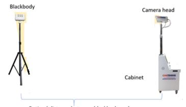
Optimal distance between blackbody and camera head is 3m (10') to 8m (26')
